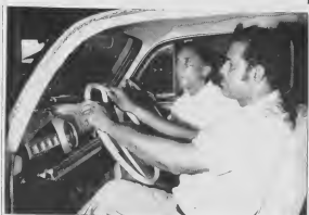
THE AUTO DRIVING SCHOOL'S classroom is the 1948 coupe as R. C. Senchin, background, the school's instructor, may assume control of the car if a student falters. Note the twin steering wheels, double sets of foot pedals.
